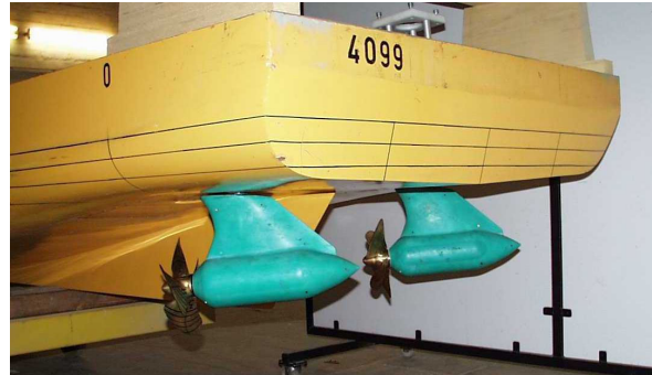
Fig. 3 Two KAMEWA-Pod-models on the model of the Cruise Liner “Millennium”
