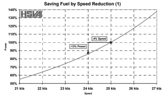
Fig. 12: Reducing the speed by 1 knot reduces the required power by 13%
