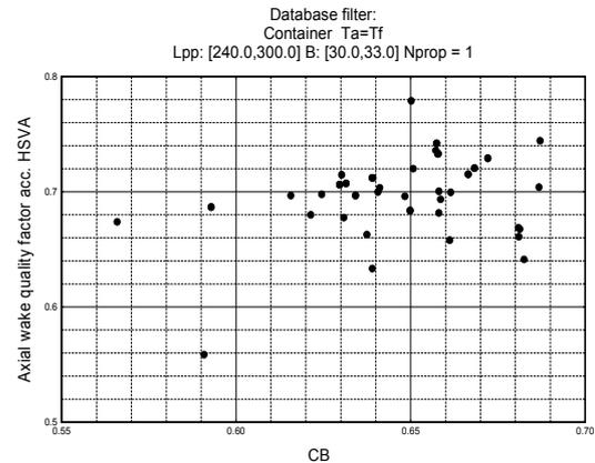
**Fig. 5: Axial Wake Quality Factor of container vessels of about 4200 TEU**
