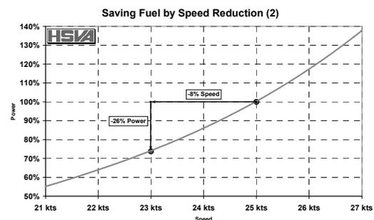
Fig. 13: Reducing the speed by 2 knots reduces the required power by 26%
