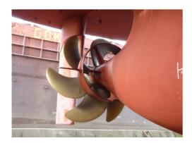
Figure 2 Becker Twisted Fin®, first installation on a 7090 TEU Container Vessel, Hamburg Süd
