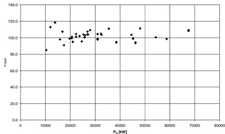
**Fig. 5.5 – Propeller Speed  $n = f(P_D)$**
