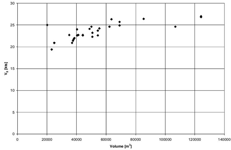
**Fig. 6.4 – Service Speed  $V_S = f(\text{Volume})$**
