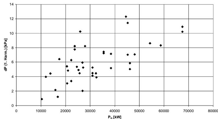
**Fig. 7.1 – Measured Pressure Pulses, 1<sup>st</sup> Harmonic**
