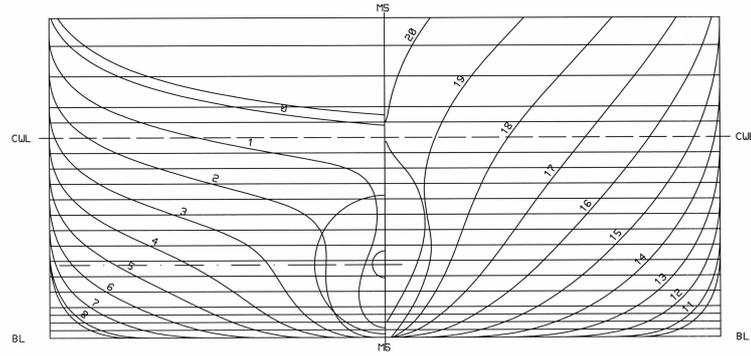
**Fig. 4.2 – Typical Hull Lines of a ULCS – 8,100 TEU**
