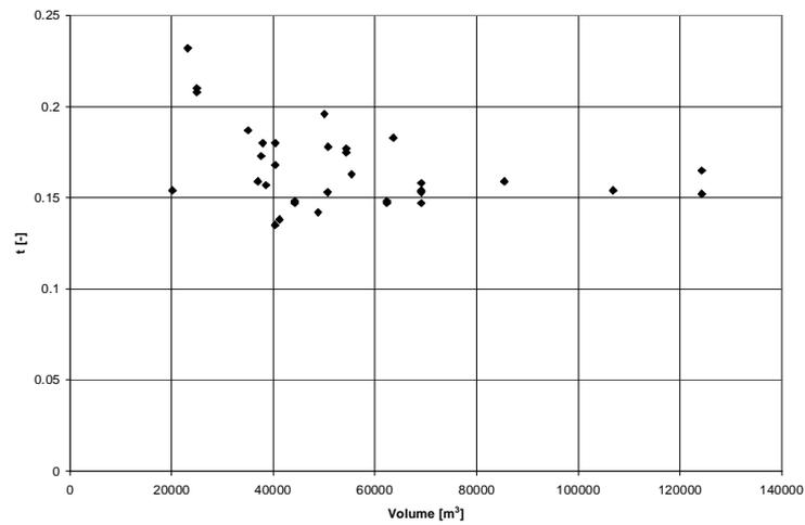
**Fig. 6.5 – Thrust Deduction Fraction at Service Speed  $t = f(\text{Volume})$**
