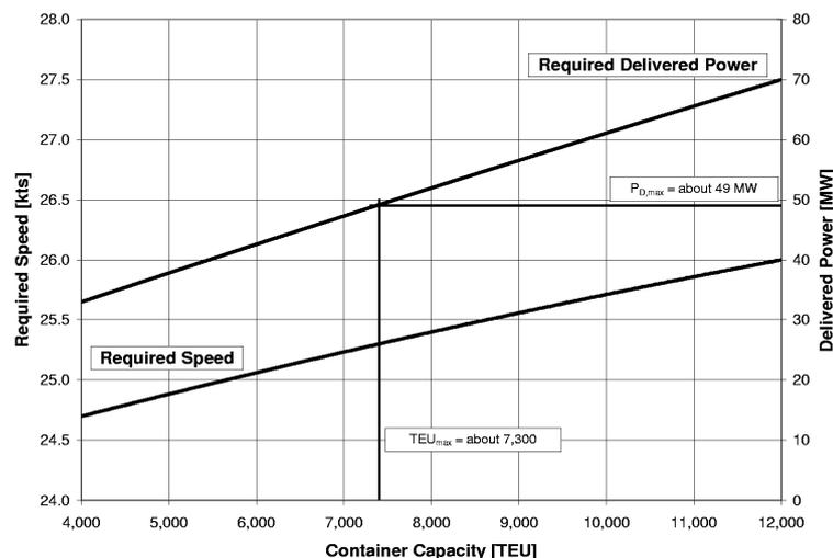
**Fig. 6.1 – Required Speed and Delivered Power for LCS**
