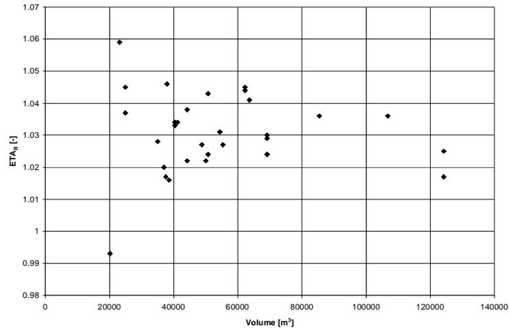
**Fig. 6.7 – Relative Rotative Efficiency at Service Speed  $\eta_R = f(\text{Volume})$**
