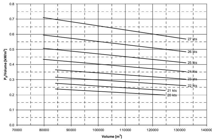
**Fig. 6.3 – Specific Power Requirement for VLCS**
