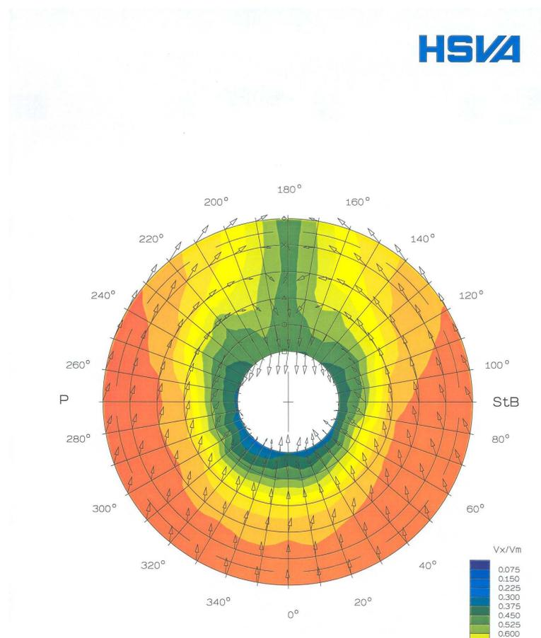
**Fig. 4.1 – Typical Wake Field of a ULCS – 8,100 TEU**
