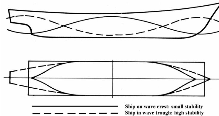
**Fig. 7.3 – Ship Stability on Wave Crest and in Wave Trough (Source: Schneekluth, 1988)**
