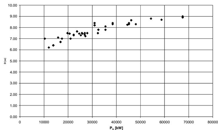
**Fig. 5.2 – Propeller Diameter  $D_p = f(P_D)$**
