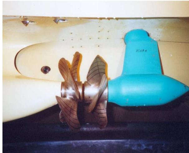
**Fig. 8.3 – Pod Drive Behind Main Propeller**
