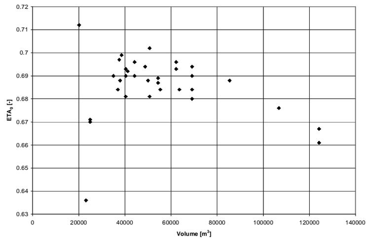
**Fig. 6.8 – Propeller Efficiency at Service Speed  $\eta_0 = f(\text{Volume})$**
