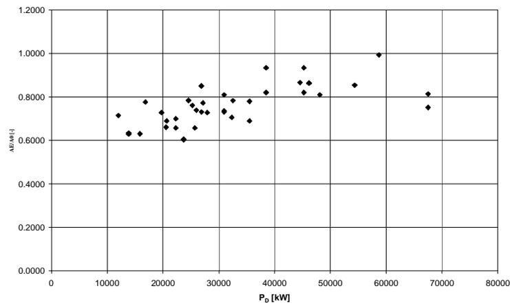
**Fig. 5.4 – Expanded Blade Area Ratio  $A_E/A_0 = f(P_D)$**
