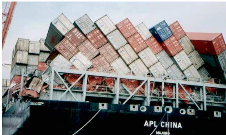
**Fig. 7.4 – Cargo Damages after Parametric Rolling**
