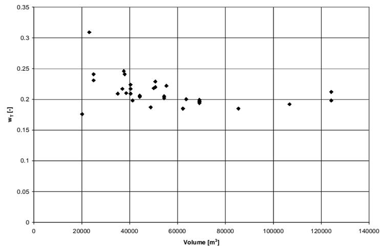
**Fig. 6.6 – Wake Fraction at Service Speed  $w_T = f(\text{Volume})$**
