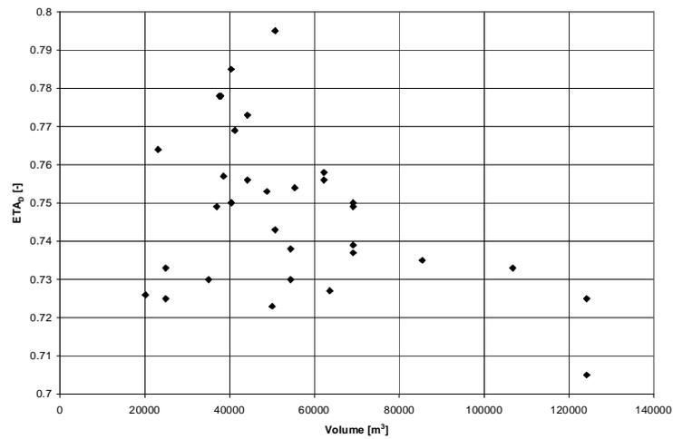
**Fig. 6.9 – Propulsive Efficiency at Service Speed  $\eta_D = f(\text{Volume})$**
