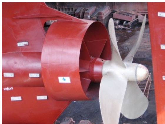
Figure 1 First installed full scale Mewis Duct®, STAR ISTIND, 54,000 DWT MPC, September 2009
