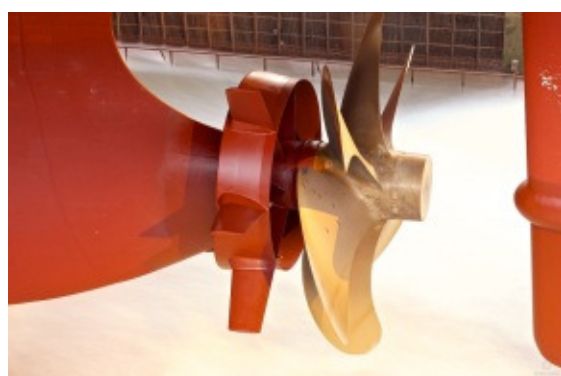
Figure 9 First installed full scale Becker Twisted Fin®, MS SANTA CATARINA, 7090 TEU CV, December 2012
