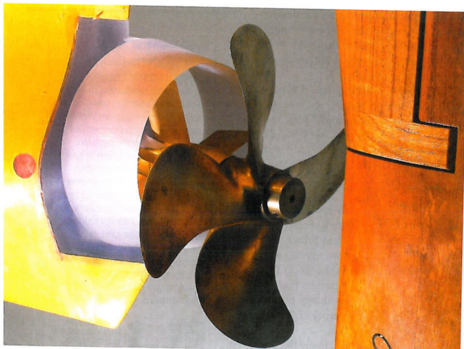
Fig. 11: Bulk carrier ship model with installed PSD model, view diagonal from the back/port
