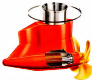
The Azipod unit incorporates an electric AC motor, located inside the pod.
