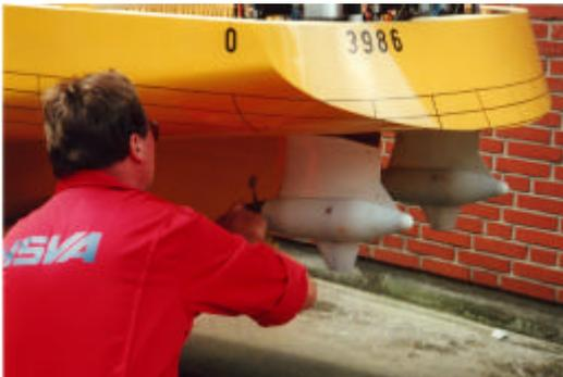
Fig. 2 Pod units installed on a twin-screw ship model
